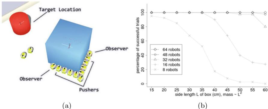
**Fig. 1.** (a) Robots that have pushed a cuboid object near to the target location. (b) Percentage of successful trials for 8, 16, 32, 48 and 64 robots transporting objects of different size/mass (40 trials per data point).
