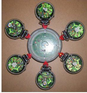
Fig. 5. Experimental setup. An object has to be transported towards a target (on the bottom; not shown). Six robot are manually attached to the object. While some robots are fully operational, others are not capable of perceiving the target.
